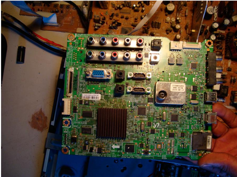
**Figure 1** Television repairman explaining the differences between ‘Compressed’ LCD circuits (the lower panel) and ‘Scattered’ tube circuits (the upper panel). Photo by the Author.
